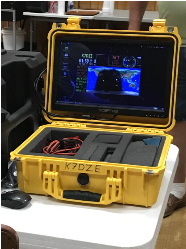
The computer is an Odroid N2 from Hardkernel running a full distribution of Ubuntu LINUX KC9MZ Photo
