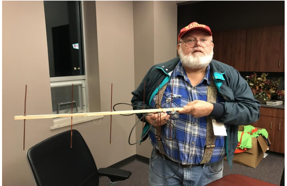
John, WA0LIS shows off his homebrew 440 Mhz YAGI antenna at the last club meeting.
