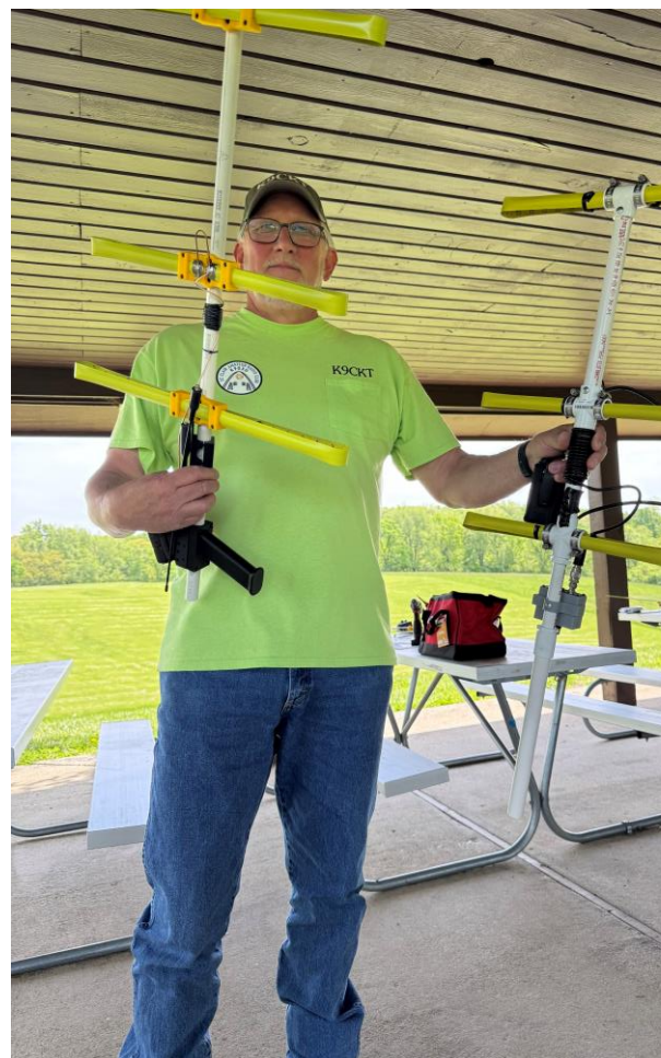
Ken shows us a couple of tape measure antennas KC9MZ photo
